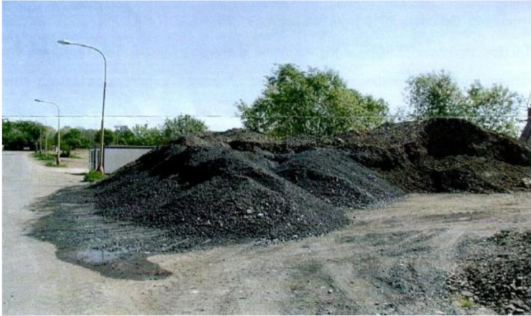
Photo 4: Interim storage of mixed fly ash and bottom ash from MWI Liberec, Czech Republic before its use as construction material in one of the municipalities. Levels of PCDD/Fs in this material are 0.05 – 0.1 ppb in WHO-TEQ.
